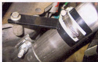
▲ Two brackets are affixed to the transmission and clamped on each side of the Y-pipe tubing, and help keep the tubing structure rigid and free of vibration against the Mustang's chassis.
