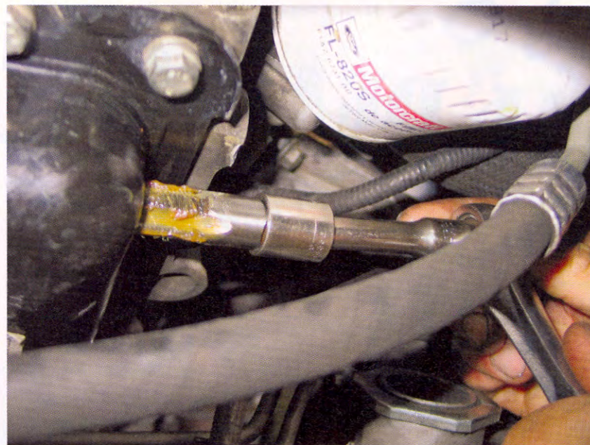
▲ On the oil side, yes, punching a hole in the pan (for a drainback line) is required. A punch and 3/8-inch NPT tapping tool are included. Note the use of thick grease on the tap, which helps keep metal shavings out of the oil pan when threads are being cut.
