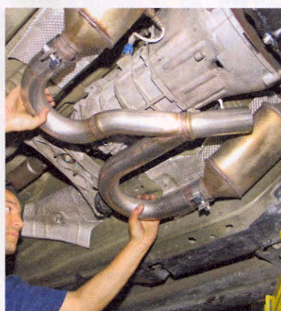
▲ The only cutting is done on the 'Stang's factory H-pipe tubing 2 1/2 inches back from the welds on each cat. With the exhaust section removed, Ricardo installs the turbo system's Y-pipe, which routes exhaust gas to the up-pipe and into the compressor housing on the turbocharger.
