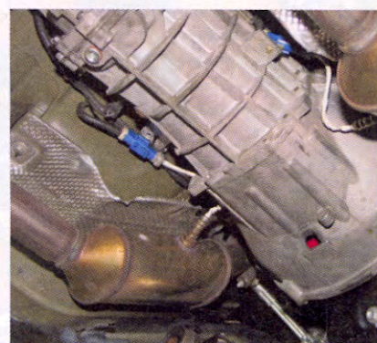
▲ These are our project 'Stang's OEM catalytic converters, which remain intact and unmodified with this CARB-legal turbo system. Despite the performance gains that come with removing these pieces and replacing them with H- or X-shaped crossover tubing, tampering with or removing cats is a huge no-no in any state. Without the converters, the Turbonetics Mustang system wouldn't stand a chance at being validated by CARB.
